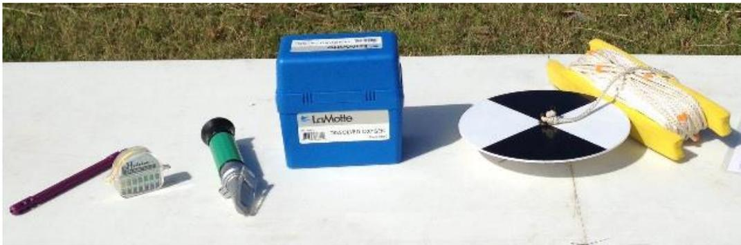
Water Quality Testing Materials (l-r): thermometer, pH paper, refractometer, LaMotte dissolved oxygen test kit, Secchi disk
