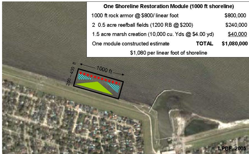
Figure 4: Dimensions and elements of a single shoreline restoration module. Costs are based on the estimated cost of rock armoring for restoration projects elsewhere along the Louisiana coast.
