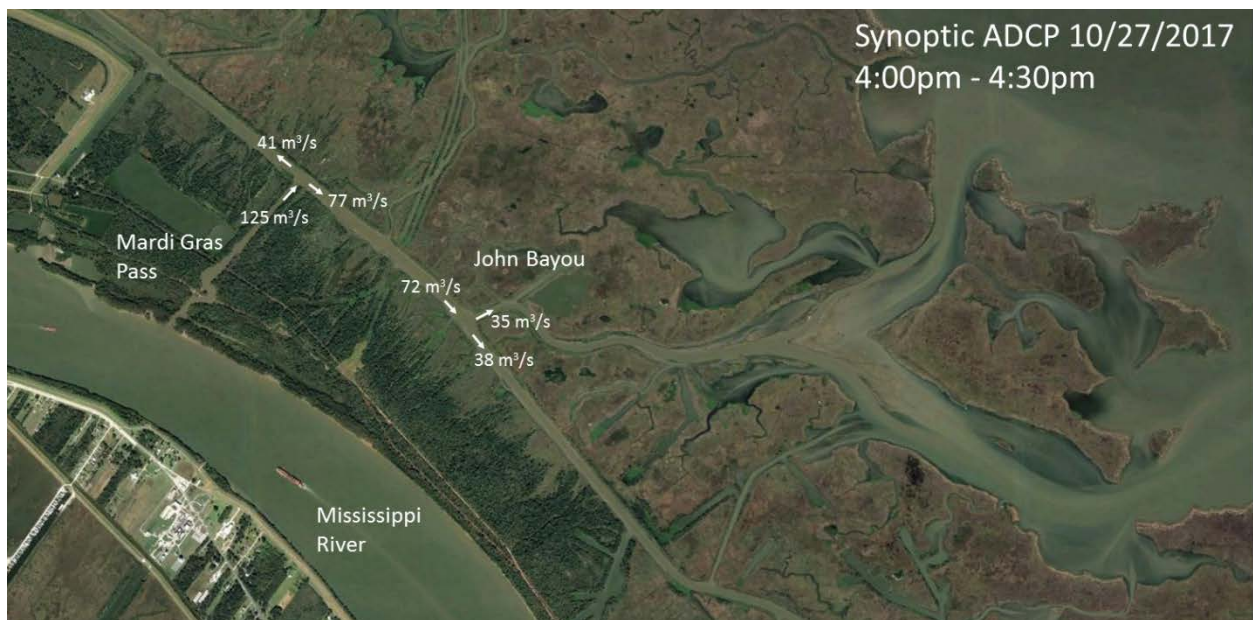
Figure 4. Mardi Gras Pass flow and flow distribution in the receiving basin at key junctions in the back levee canal and John Bayou.
